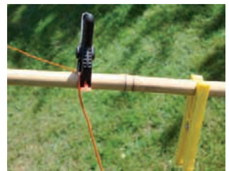
Fig. 5: to variations of the method of temporarily fixing a loop element to the spreaders during the tuning and adjusting phase.
